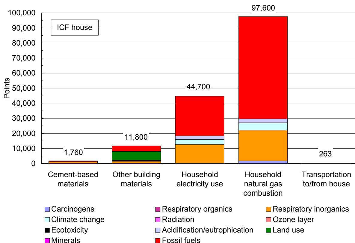
**Figure 3. Single-score life cycle inventory assessment of ICF house in Chicago showing contribution of each major process/product stage (output from SimaPro). The data have been normalized and weighted according to the Eco-Indicator 99 method using the Egalitarian perspective.**
