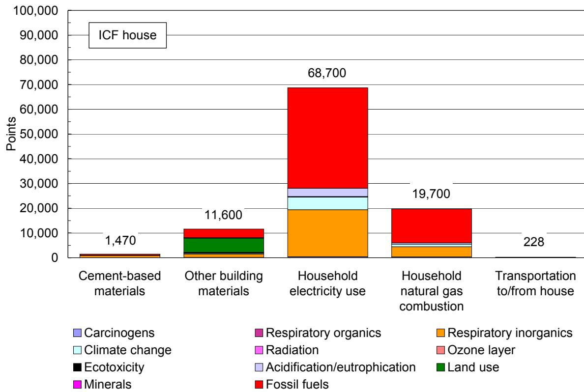
**Figure 2. Single-score life cycle inventory assessment of ICF house in Miami showing contribution of each major process/product stage (output from SimaPro). The data have been normalized and weighted according to the Eco-Indicator 99 method using the Egalitarian perspective.**
