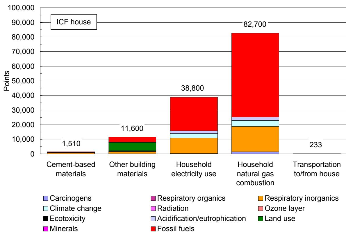
**Figure J-2. Single-score life cycle inventory assessment of ICF house in Seattle showing contribution of each major process/product stage (output from SimaPro). The data have been normalized and weighted according to the Eco-Indicator 99 method using the Egalitarian perspective.**
