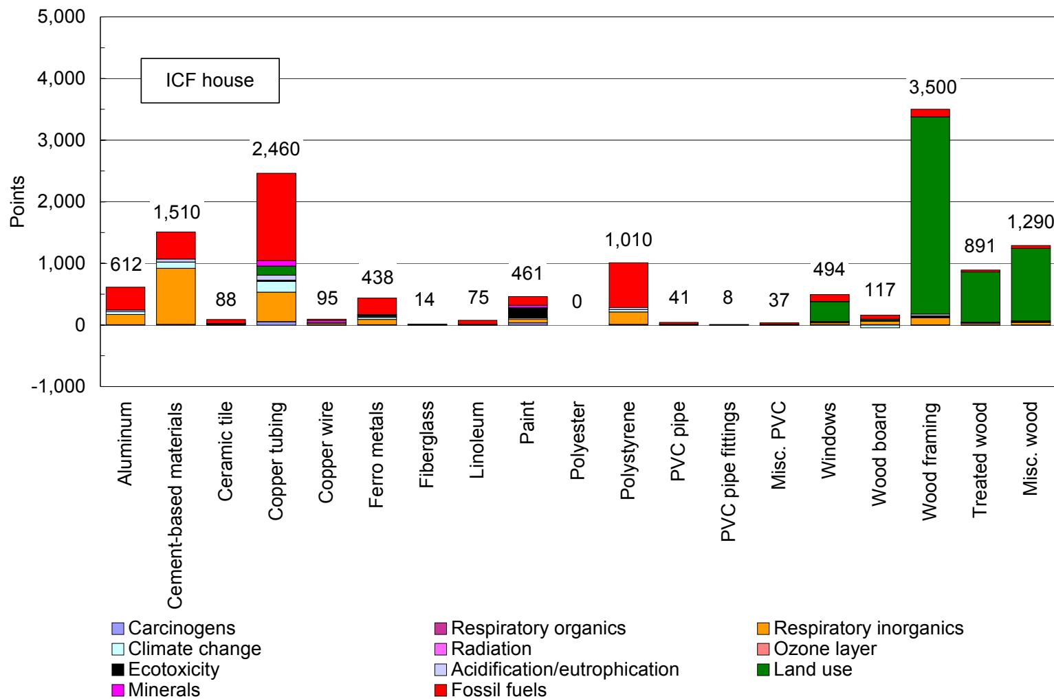
**Figure K-2. Single-score life cycle inventory assessment for construction materials in the ICF house in Phoenix (output from SimaPro).**
