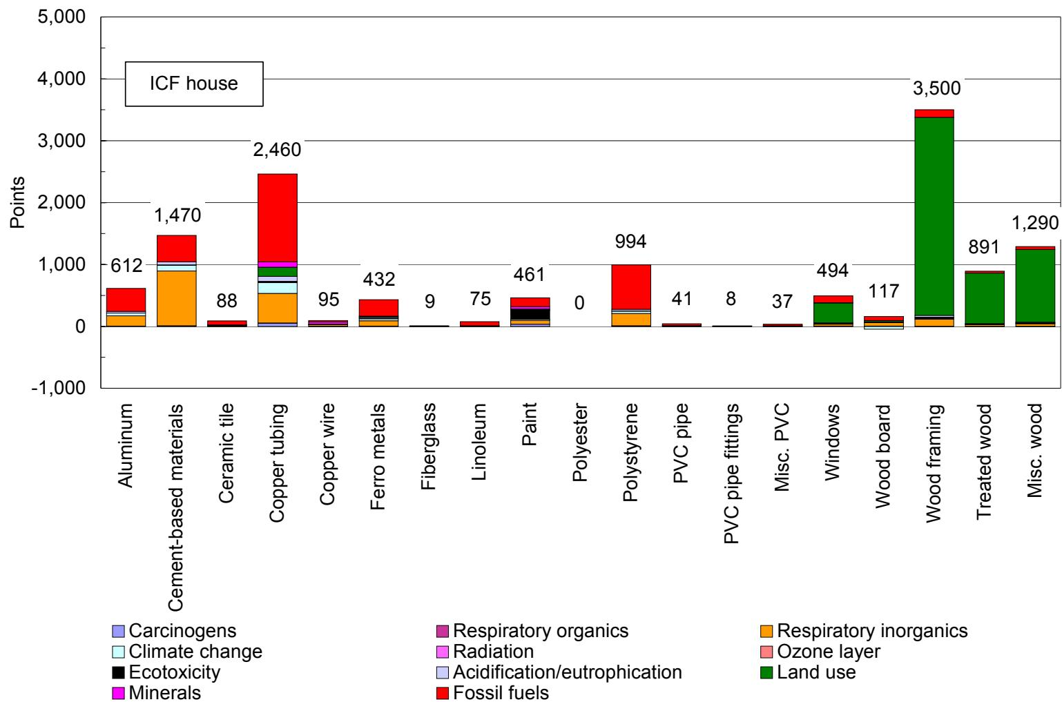
**Figure K-1. Single-score life cycle inventory assessment for construction materials in the ICF house in Miami (output from SimaPro).**
